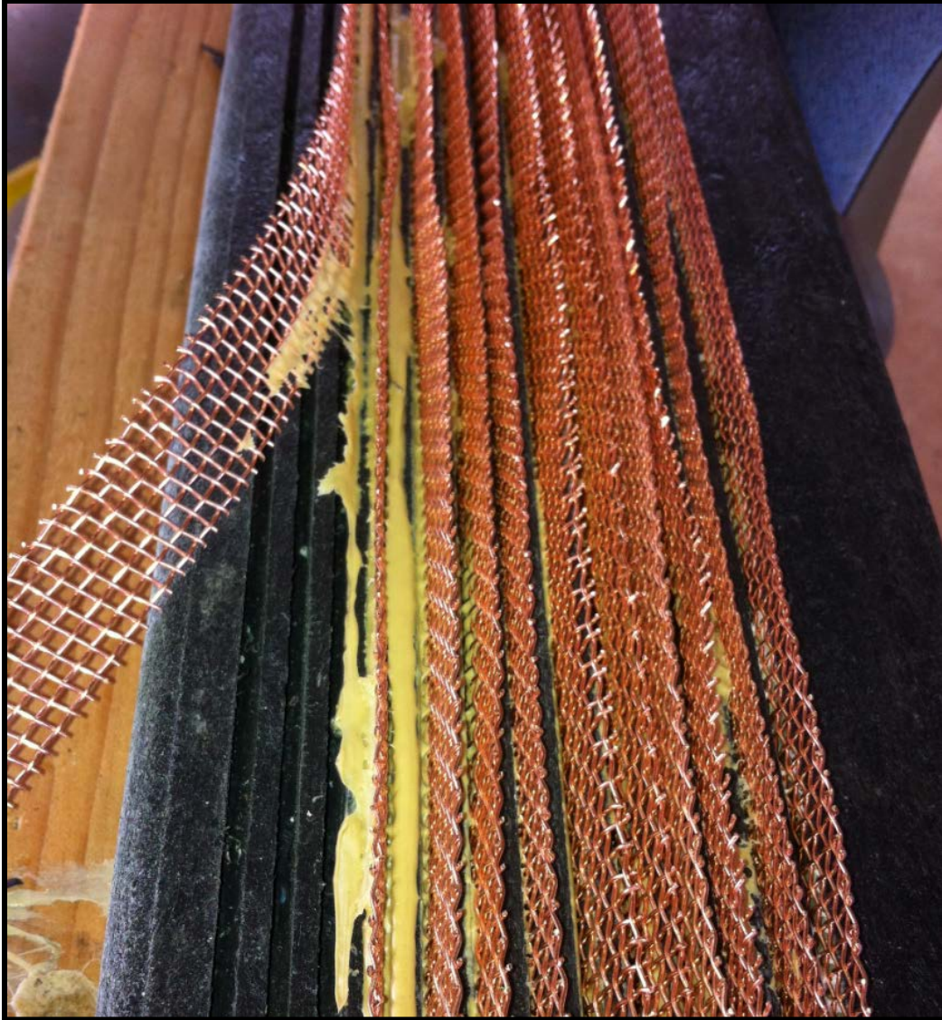
Figure 5. Partially completed cut mesh board, ten grooves filled with copper mesh and three remaining.
